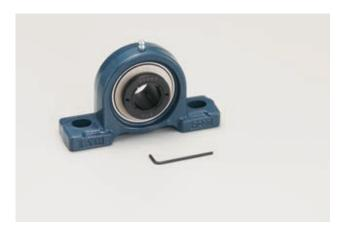
Tighten the set screws by hand. Tightening the set screws creates extreme holding power over traditional adaptor sleeves without any change to the bearing clearance.
